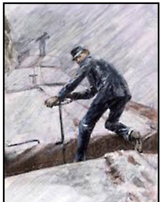
Before automatic air brakes the brakeman would go from car to car setting brakes manually.
