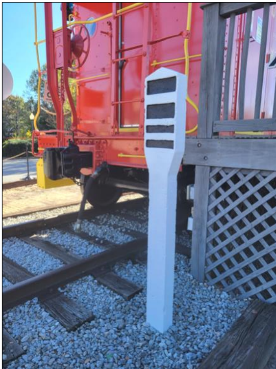
Newly installed whistle post at the caboose. Notice that the two longs and two shorts are different than used today. "The road crossing signal two longs and two shorts was adopted as Rule 49 on April 14, 1887 by the General Time Convention. On April 12, 1899 the same signal became Rule 14(l) in the completed Standard Code of Operating Rules that was adopted by the General Time Convention. It remained that way until November 1938, when it was changed to two longs a short and a long, prolonged or repeated until the crossing is reached."
