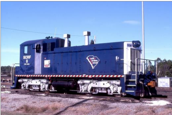
One of the South Carolina Central's few switchers, SW1200r #8, is seen here in Hamlet, North Carolina during April of 1998.
