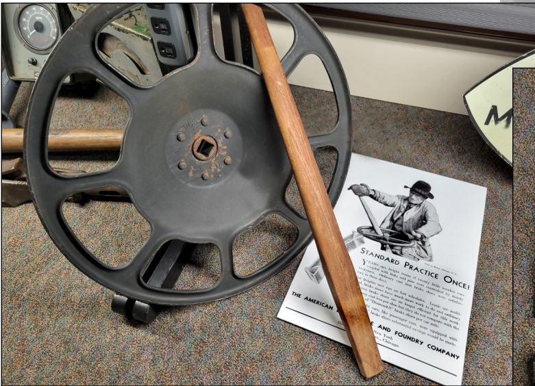
↑ Old time brake club used to hand tighten a cars brakes. These photos show some of the new displays in the museum.
