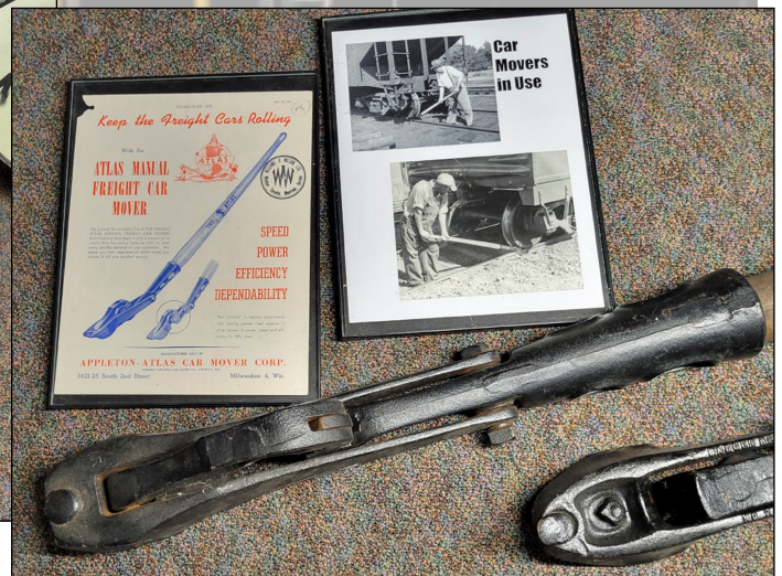
↑ Hand powered car mover used to manually spot a car.
