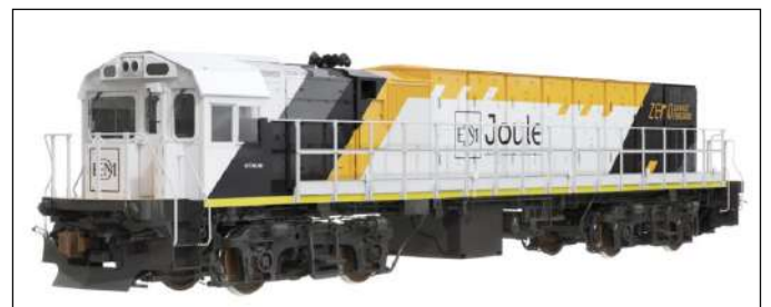
↓ Progress Rail "Joule" battery electric locomotive.
