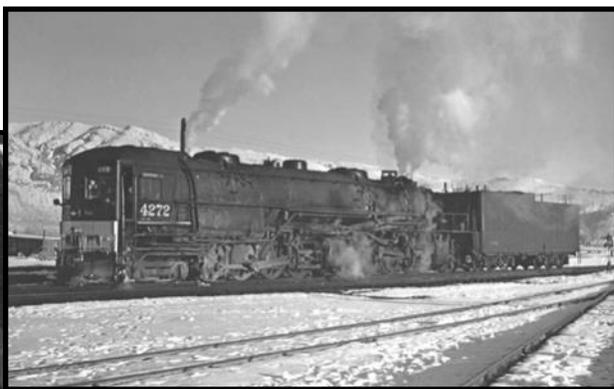
↑ The cab forward locomotive was developed to put the crew in front of the exhaust.
