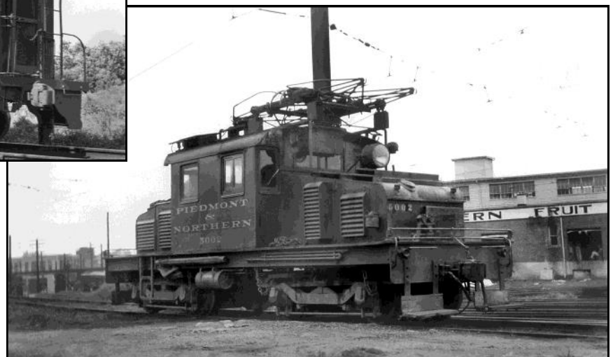
P&N #5002 built by Baldwin-Westinghouse in 1911-12 with two trolley poles and refitted in 1935 with a pantograph.
