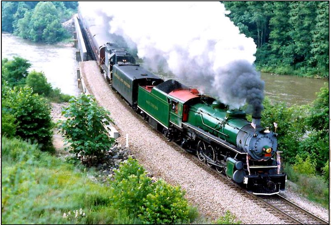
Southern Railway locomotive #4501, a 2-8-2 Mikado type, on a fan trip in Tennessee.
