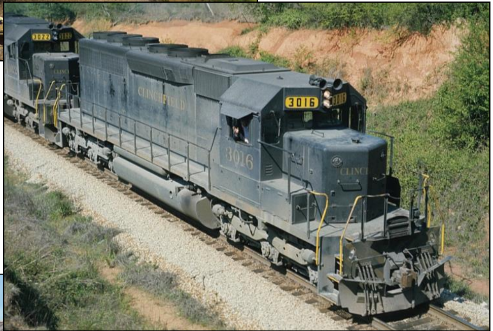
An EMD SD-45 in a cut at Spartanburg, SC. The weathering shows the hard mountain use these units received.
