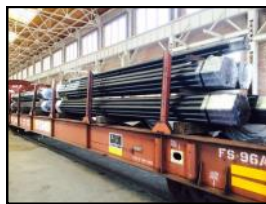
New flues for the 611.
