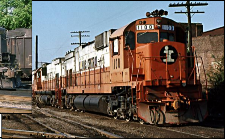
Illinois Central #1100—an ALCO C-636. Although built in the late 1960s it is representative of the motive power used in the 1970s from ALCO.
