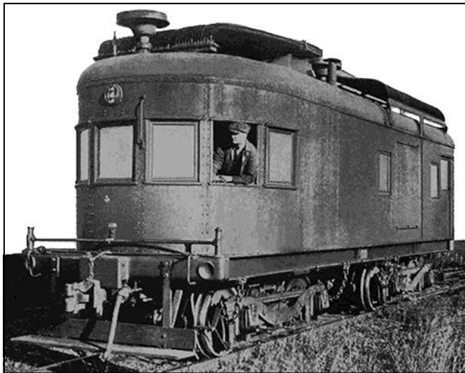
Early GE-IR diesel, above is the front view - below is the rear view. Parts from earlier prototypes were used in the construction.
