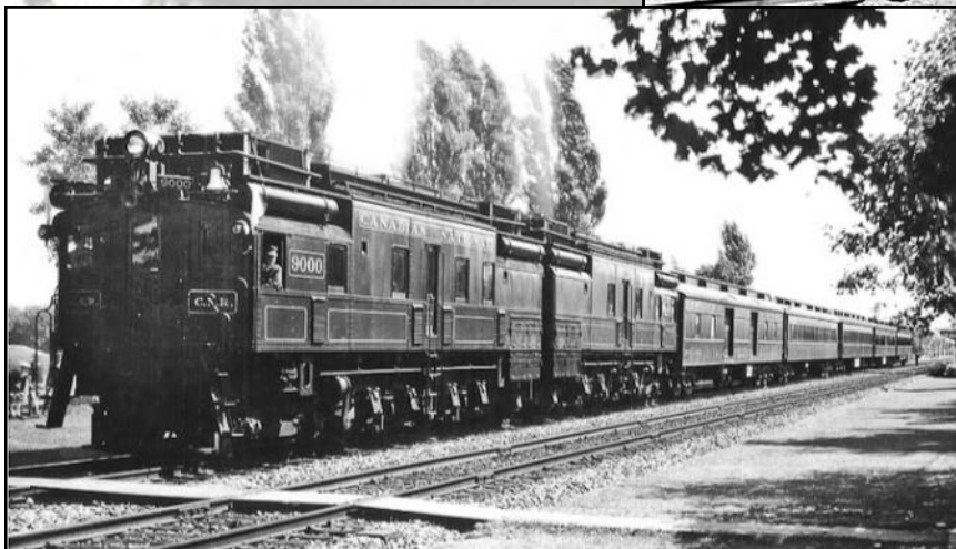
70 ton Westinghouse Visibility Cab 400 hp Beardmore diesel. CLC 1861 5/1929 It was sent to Canadian Westinghouse in Hamilton for electrical work and delivered to CNR 5/17/1930.
