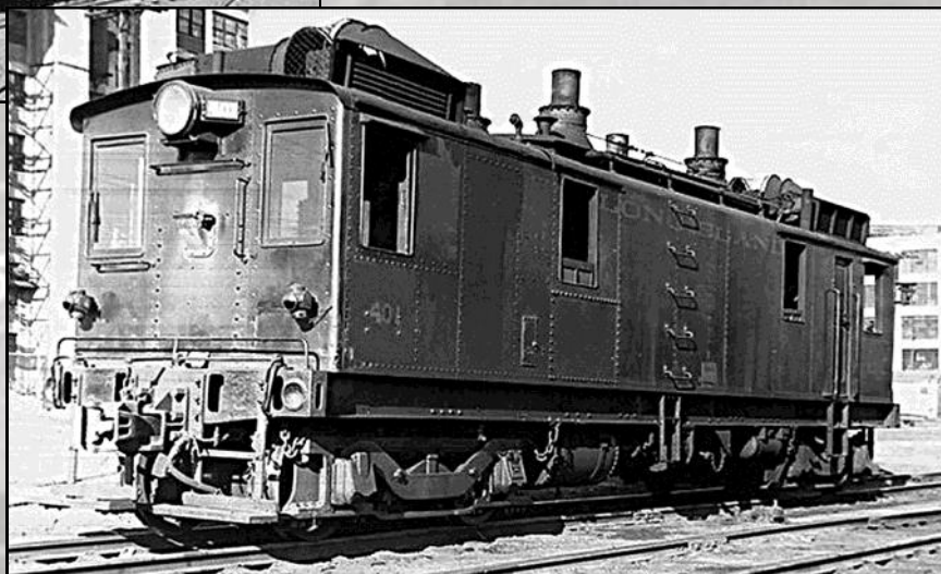
Long Island Railroad #401 a 100T locomotive. Ingersoll-Rand marketed the AGEIR locomotives in three categories. A 60 ton 300 horsepower design, 100 ton 600 horsepower version, and a 108 ton 750 horsepower unit. All three were offered in both a "Switching Service" and "Road Service" version with only a change in gear ratio to distinguish between them.
