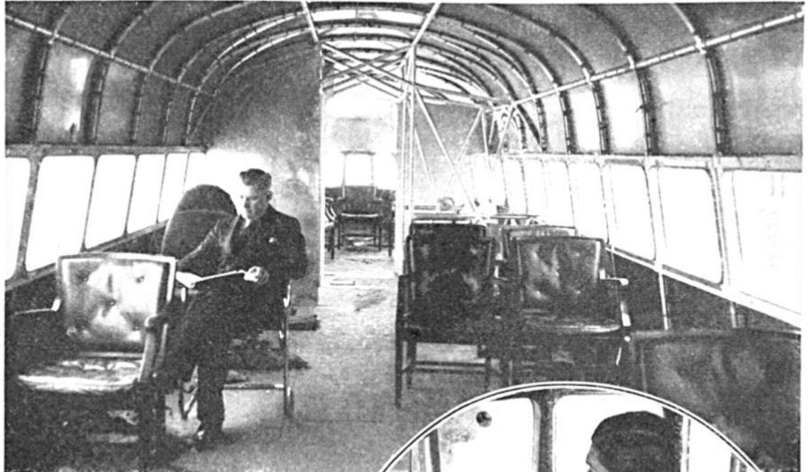
Top: Interior of Railplane before installation of soundproofing, insulating, and decorative materials. Right: Neat instrument panel resembling that of airplane cockpit.
