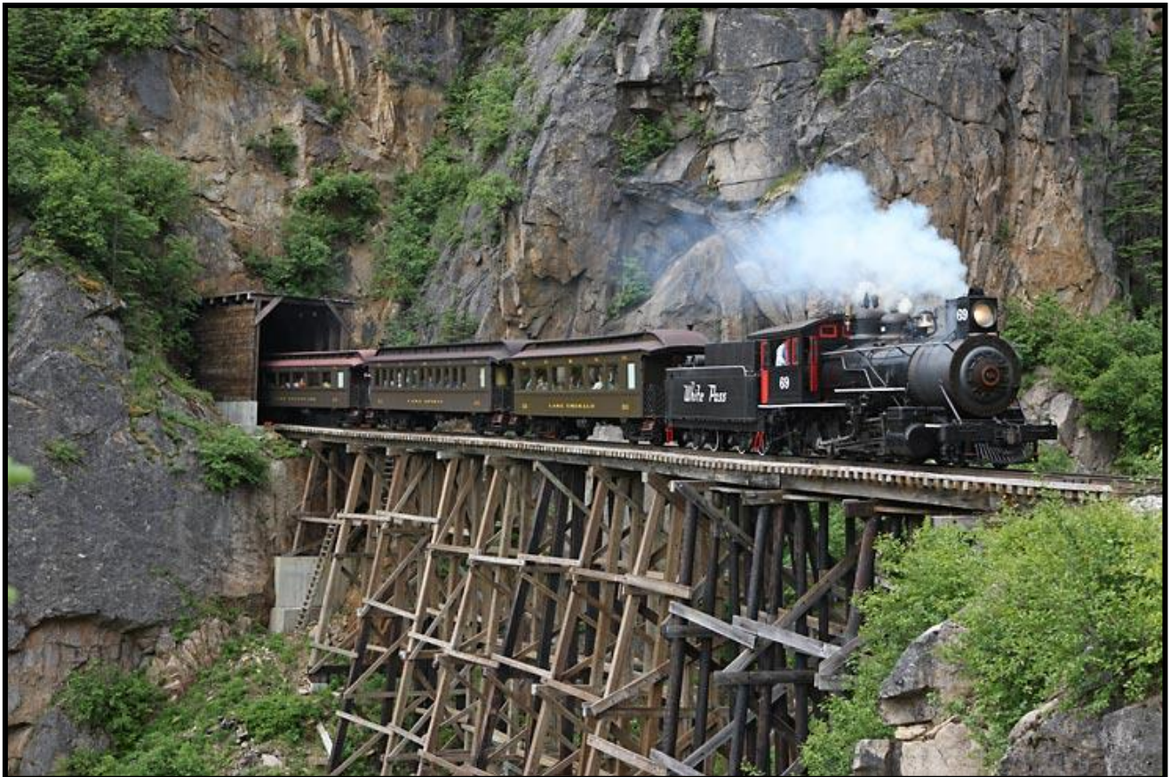
WP&Y RR locomotive #69 pulls a excursion train across a wooden trestle immediately after exiting a tunnel.
