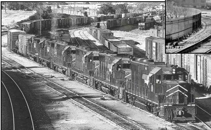
Multiple locomotives of steam required a crew for each locomotive while the multi-unit diesel locomotives can be run by one crew no matter the number needed to pull the train.
