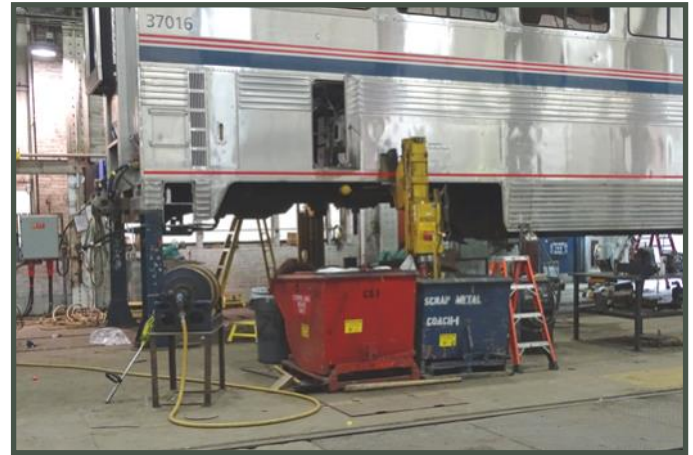
Top to Bottom: Passenger car truck removed for maintenance. Wheel turning lathe. Tour group. Locomotive shop area with special paint job on loco.
