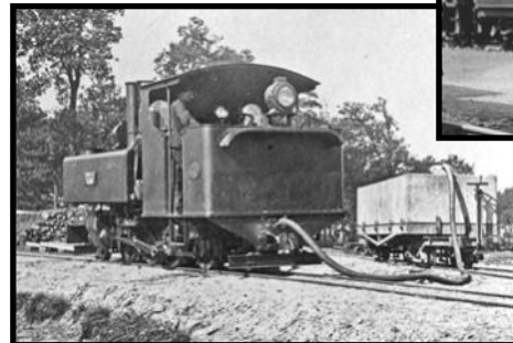
Baldwin built standard "War Dept." 4-6-0 narrow gauge trench locomotive.
