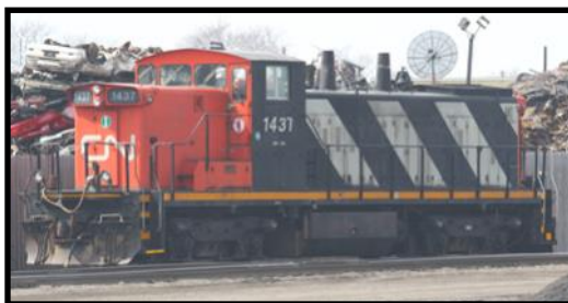
GMD-1 Canadian National switcher locomotive.
