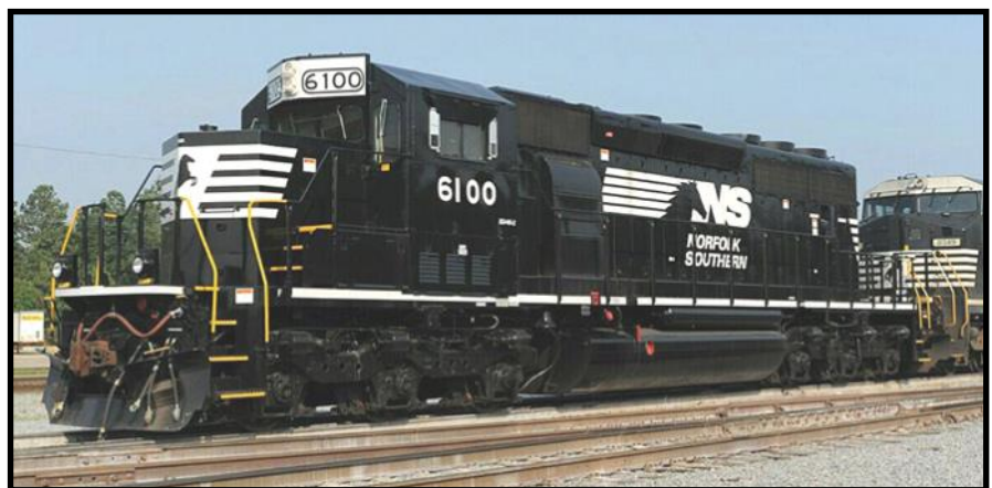
NS #6100 an EMD SD40-2 with upgrades including the "Admiral" cab.
