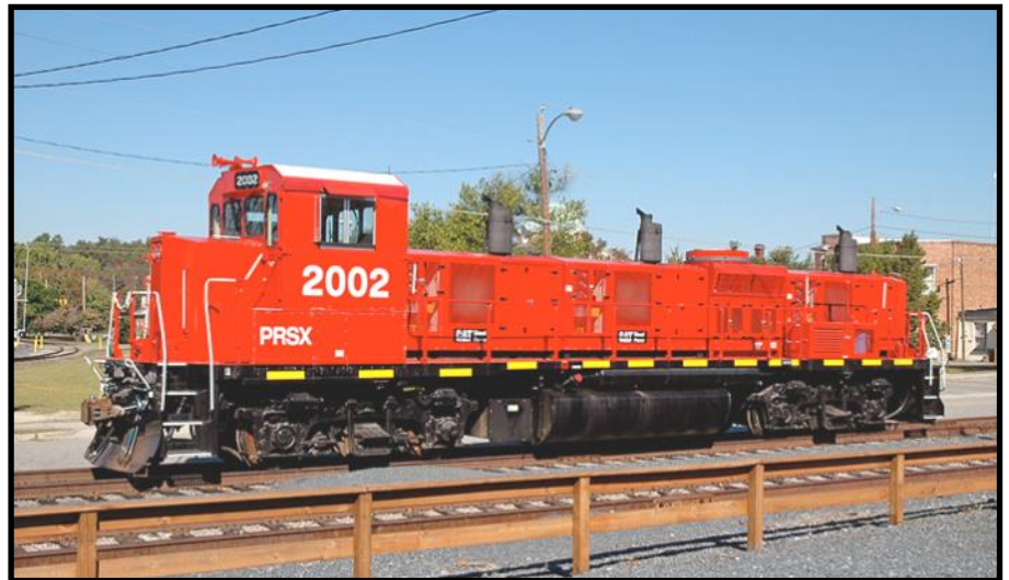
Progress Rail Genset locomotive model PR22B three motors & three generators.
