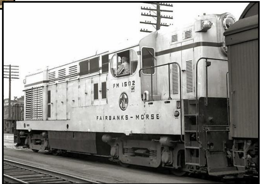
Fairbanks-Morse demonstrator #1502 a H-15-44 model road switcher.
