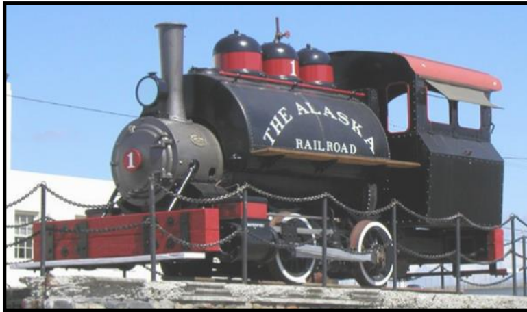
Davenport loco built narrow gauge for Panama Canal construction and later converted to standard gauge for Alaska Railroad, now restored and on display.
