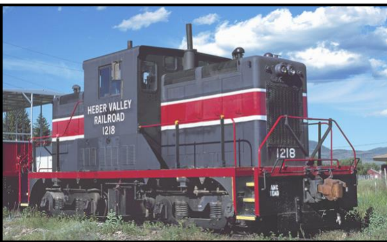
A restored Davenport 44-tonner on the Heber Valley Railroad.
