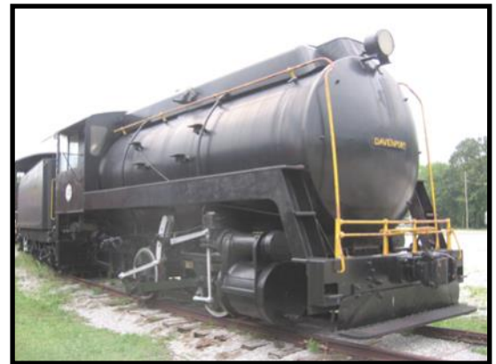
A fireless "cooker" industrial locomotive.
