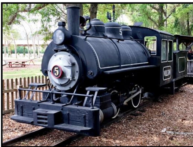
Vulcan's early "bread and butter" size locomotive was the small industrial steam locomotive—0-4-0T and 0-6-0T's. Loco is on display at Tifton, GA.
