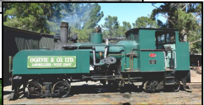
Heisler design built in Australia, note the British influence on cab and water tank.
