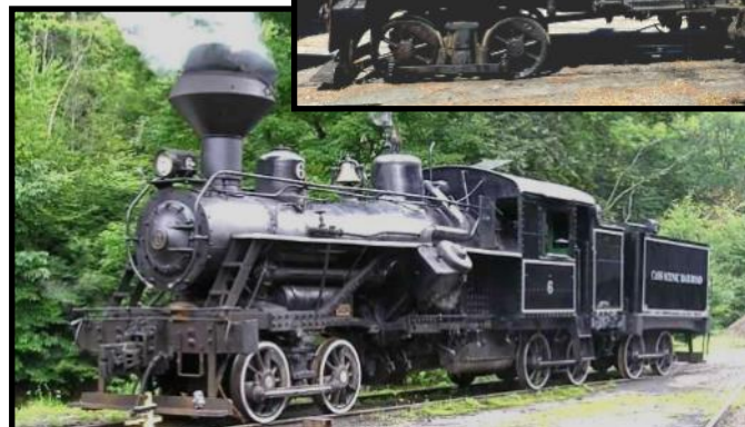
Heisler design built in Australia, note the British influence on cab and water tank.
