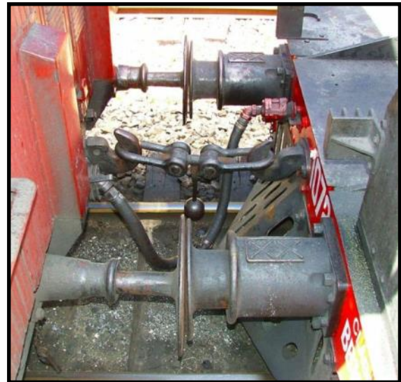
Screw-tensioned three-link coupling. The narrow buffers of the left-hand vehicle are sprung, the thicker buffers on the right contain a hydraulic damper. Typically European in use.
