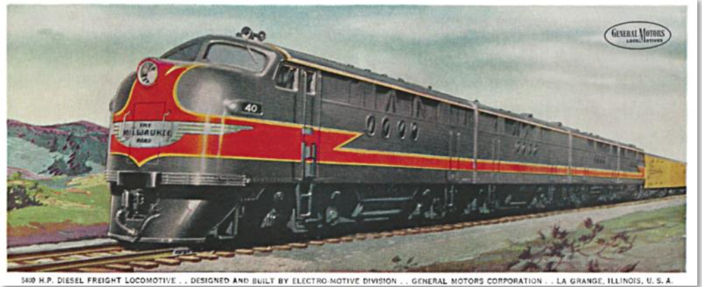
3400 H.P. DIESEL FREIGHT LOCOMOTIVE . . . DESIGNED AND BUILT BY ELECTRO-MOTIVE DIVISION . . . GENERAL MOTORS CORPORATION . . . LA GRANGE, ILLINOIS, U. S. A.
