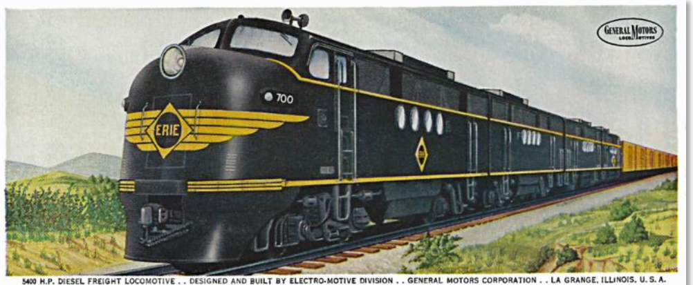
5400 H.P. DIESEL FREIGHT LOCOMOTIVE . . . DESIGNED AND BUILT BY ELECTRO-MOTIVE DIVISION . . . GENERAL MOTORS CORPORATION . . . LA GRANGE, ILLINOIS, U. S. A.
