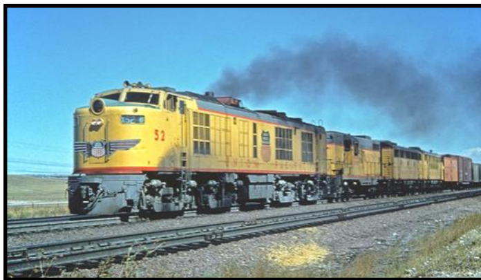
From January 1952 to August 1953, UP received units 51-60, like the prototype but with a cab at only one end to increase fuel capacity. Each cost US$540,000.
