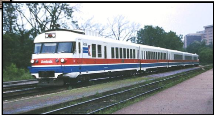
The RTG (from the French Rame à Turbine à Gaz , or gas turbine train) model was an Americanized version of the French ANF T 2000 RTG Turbo train.
