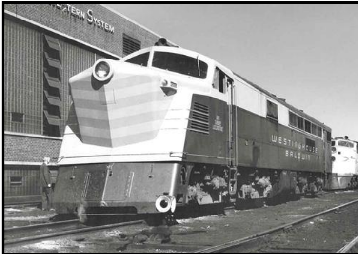
Westinghouse-Baldwin No. 4000 was an experimental 4,000-hp B-B-B-B demonstrator locomotive built in 1950.
