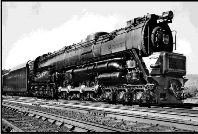
The PRR #6200 6-8-6 direct drive steam turbine locomotive was a one-of-a-kind and even sprouted "elephant ears" at one point.
