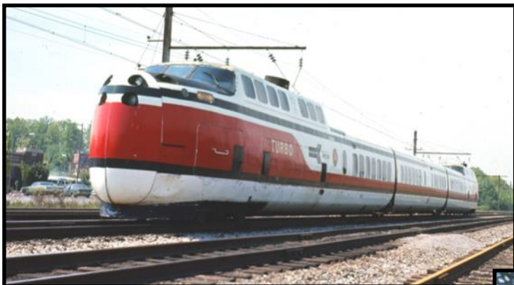
The United Aircraft Corp. built one of the first gas turbine powered trains to enter service for passenger service.
