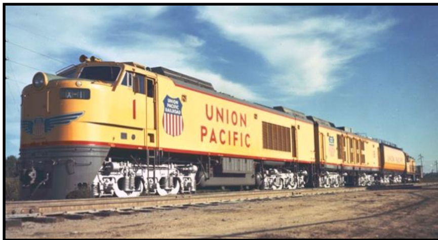
Early General Electric Gas Turbine built for the Union Pacific.
