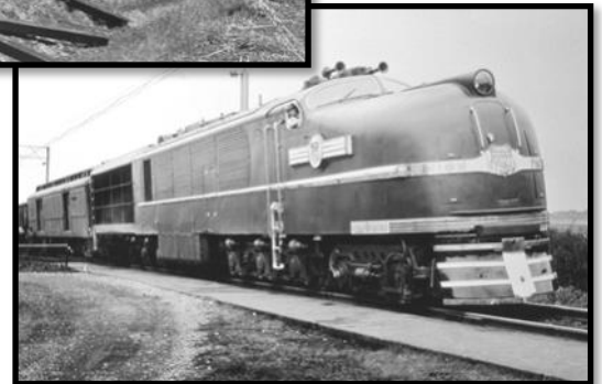
Photo of the Union Pacific GE steam turbine locomotives, April 1939. Photo at right shows the loco with an unusual dark paint scheme.
