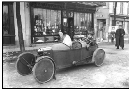
A Cyclecar is a small, lightweight, inexpensive means of transportation., between a motorcycle and full size automobile.
