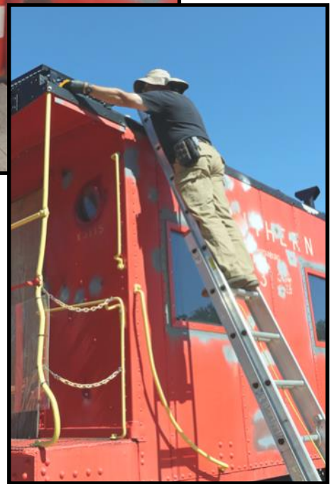
Volunteer → help applying sealer to seams on the roof.
