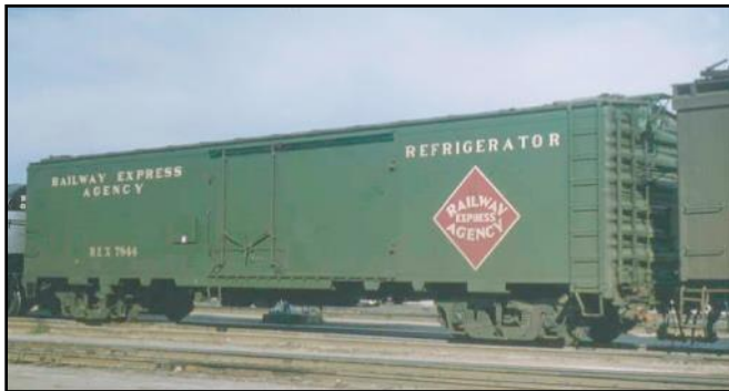
REA had express box and reefer cars made to run at passenger train speeds.
