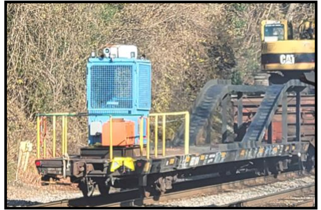
↑ Operator car for reverse moves and excavator carrier. ← Georgetown Rail Equipment locomotive pulling a old tie removal train. Sounded like a GP-9.
