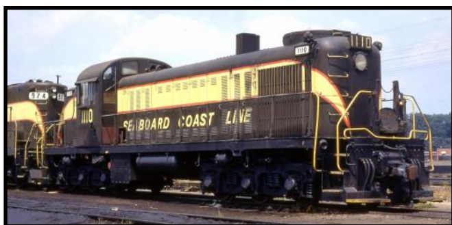
Seaboard Coast Line #1110, Alco RSC-3, 12-244, 1600 HP, 99 of these units were built in 1950-55.
