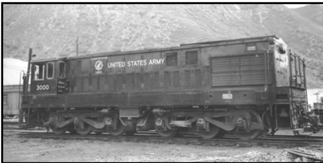
GE multi-gauge locomotive originally built for operations in Alaska in the Durango yard.
