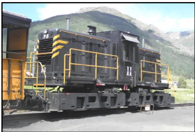
D&SNG #11 a U.S. Steel shop built loco from GE parts.
