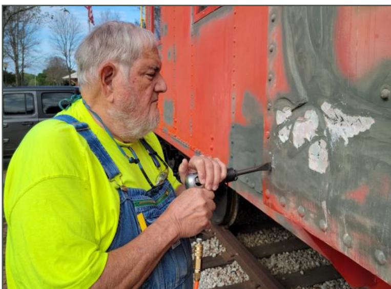
Pat O'Shields removes water damaged Bondo to reveal some damage the caboose received while in service.
