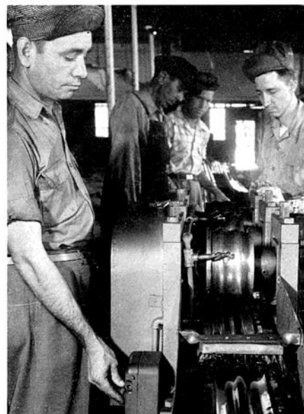
STAINLESS STEEL fluting is straightened in this motor-operated roller developed at the Hayne Shop.
