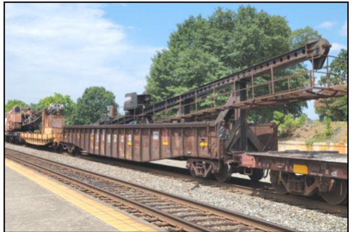
← An old N&W pile driver on a passing freight train. It was in two parts: the crane with the boom and the driver portion. ↑
