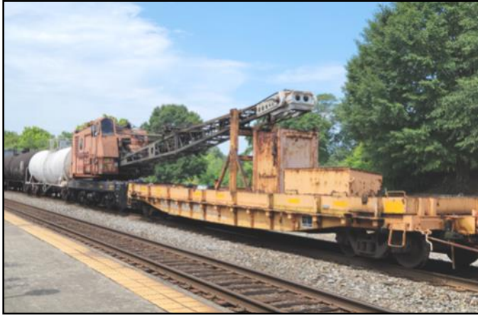
← An old N&W pile driver on a passing freight train. It was in two parts: the crane with the boom and the driver portion. ↑
