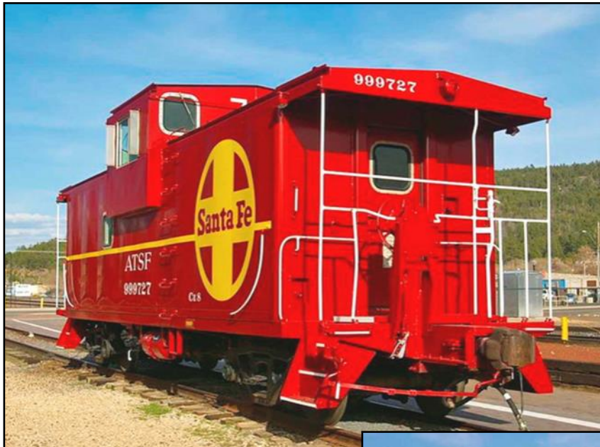
The extended vision caboose offered both the advantages of the cupola and bay window cabooses.
