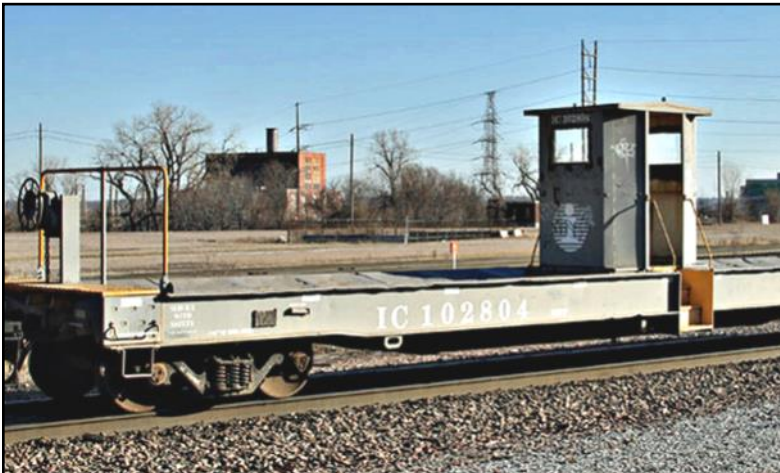
↓ An unusual transfer caboose with minimal crew quarters.
