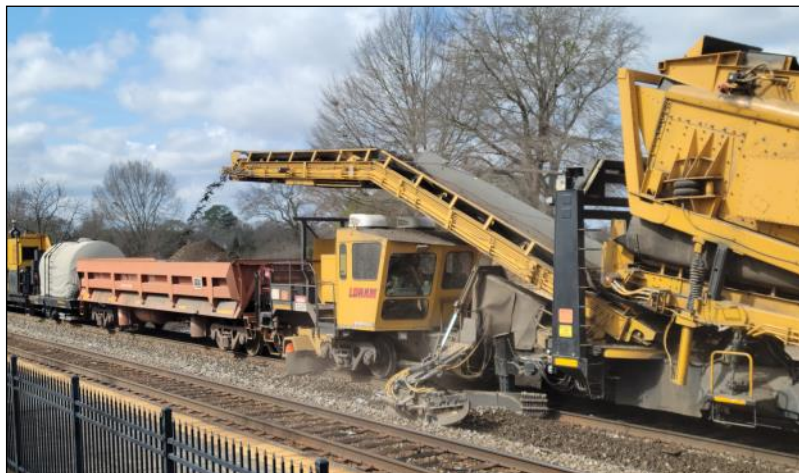
Ballast cleaning machine passing the caboose.
