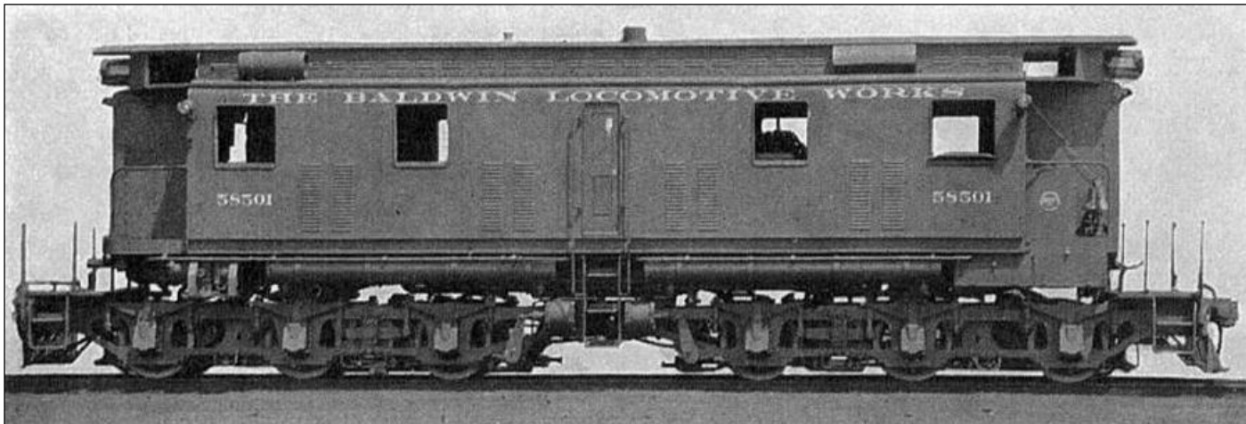
1925 Baldwin's first diesel locomotive. It was a twin engined failure.
