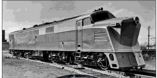
Baldwin-Westinghouse #4000, an experimental 4000hp gas turbine electric locomotive. Built in 1950.
