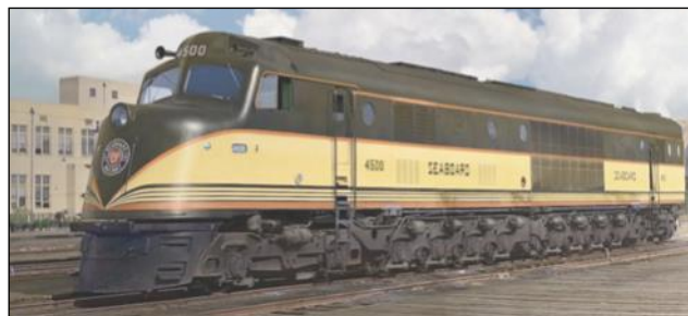
The DR-4-4-15s' whose 2-D+D-2 wheel arrangement earned the model the nickname "Centipede."
