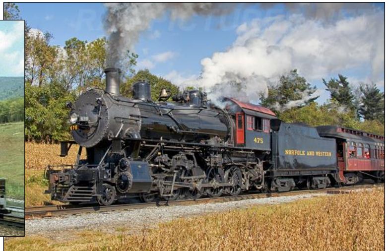
Norfolk and Western #475 is a 4-8-0 "Mastodon" type steam locomotive built by the Baldwin Locomotive Works in June 1906 .
