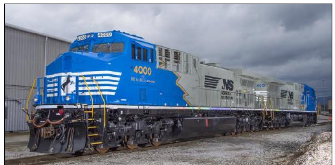
Norfolk Southern No. 4000 is a AC44C6M locomotive converted from No. 8799 a D9-40C unit built by GE in 1995.
