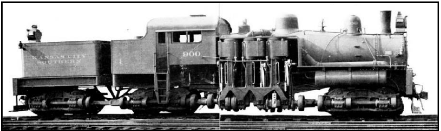
The largest and most powerful Shay geared locomotive in service.
