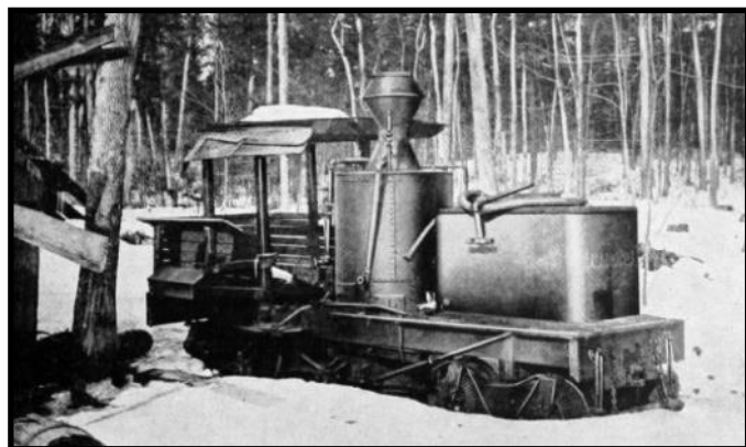
The "M. J. BOND", one of the earliest Shay locomotives built to Ephraim Shay's design by Lima Locomotive for logging in the Michigan woods.
